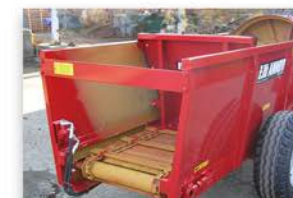
Sponda posteriore mobile ad avanzamento automatico Rear door advancing pushing manure to the turbine
